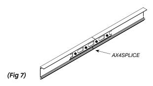
**NOTE:** Splice plates can slide completely into the channel bosses and then slide into the adjoining section after the ledge is aligned. This will aid splice plate connections for the last piece.
