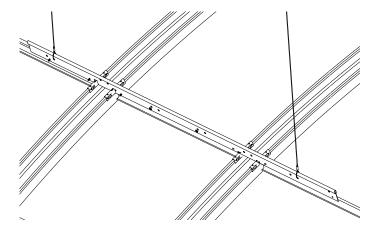
Panel lengths of 6' and 8' will have two rows of support hangers. Ten and 12' panels will require 3 rows of support hangers.
