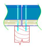
TECTUM III, E, AND NS DECKS USE TRUFAST SCREWS OR DEKFAST #14 SCREWS WITH  $1\frac{1}{2}$ " WASHER. MINIMUM LENGTH IS ONE INCH LONGER THAN PANEL THICKNESS.  $1\frac{1}{2}$ " PENETRATION PREFERRED.
