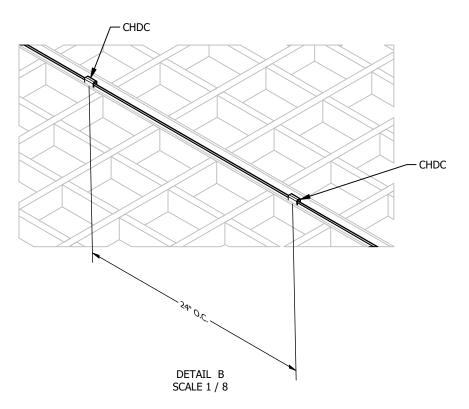
WOODWORKS OPEN CELL CLEAR HOLD DOWN CLIP (CHDC) PLACEMENT ON GRID
