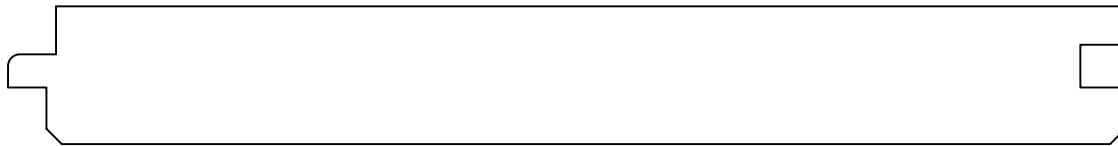
6" BEVELED EDGE PROFILE PLANK DETAIL SCALE 1 : 1
