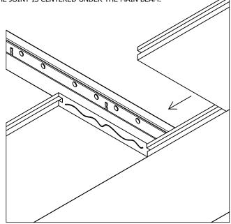
3) SLIDE EACH OF THE INSTALLED PLANK CLIPS INTO THE GROOVE OF THE PLANK.
