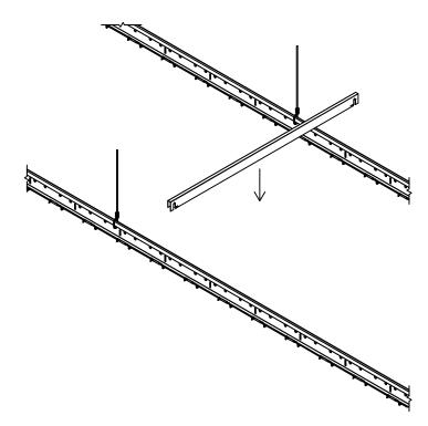
4) AS PLANKS INSTALLATION PROGRESSES, REMOVE STABILIZER BARS AND RE-USE THEM WHERE NEEDED  $\,$
