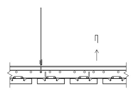
WOODWORKS LINEAR VENEERED OPEN PLANKS INSTALLATION TO LINEAR CARRIERS GUIDE
