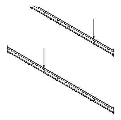
3) INSTALL PLANKS TO LINEAR CARRIERS BY ATTACHING GROOVES OF PLANKS TO FACTORY APPLIED CLIPS ON CARRIERS
