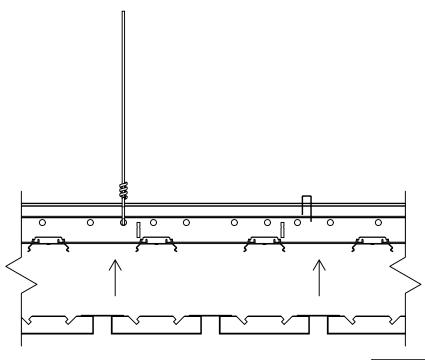
2) INSTALL STABILIZER BARS ON TO BULBS OF LINEAR CARRIERS TO KEEP CARRIERS ALIGNED. SPACE STABILIZER BARS 6' O.C. ALONG LENGTH OF CARRIERS
