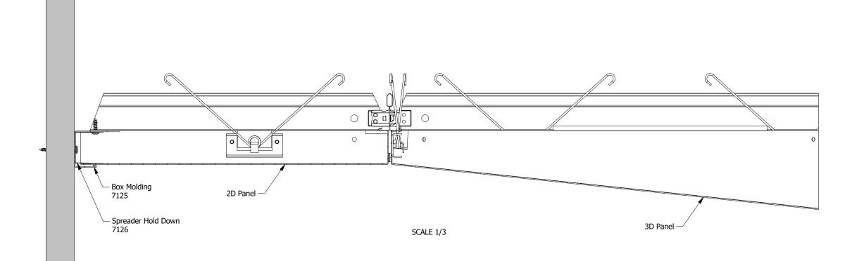
MetalWorks Torsion Spring Shapes 213787-13 3D Panel to Perimeter Detail
