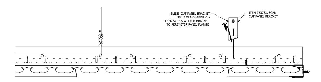
INSTALLING SYNCHRO CUT PANEL BRACKET FOR LAST PERIMETER ROW SCALE 1 / 2.5  $\,$
