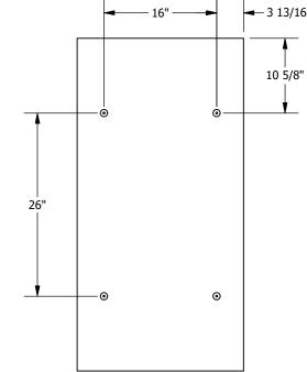
Magnet Layout - Non-Seismic Ceiling Installations
