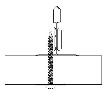
FeltWorks Acoustical Panels Screw & Washer - Installation Details
