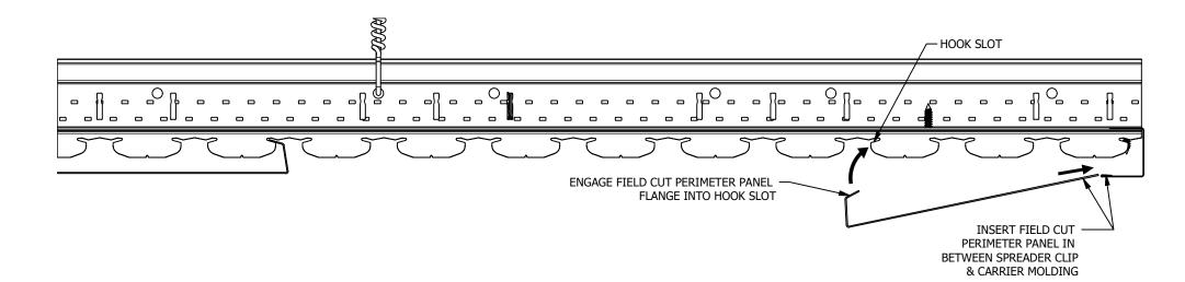
INSTALLATION SYNCHRO PANELS LAST ROW, SPREADER HOLD DOWN SCALE 1 / 2.5
