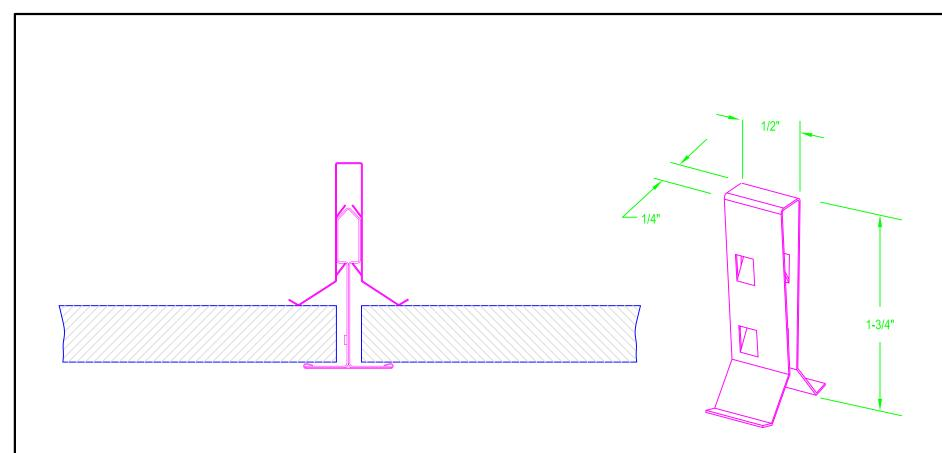
NOTE: COMPATIBLE WITH CEILING PANELS 1/16" TO 3/4" THICK.
