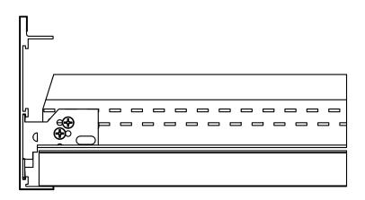
4.5.4 Attaching the Trim - Linear and Channeled The Face of the grid must be held  $\frac{7}{8}$ " above the lower flange of the perimeter trim. Use the modified twist clip (#5948) at each location where grid interfaces with the trim. Install the clips with screws or pop-rivets as shown.
